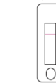
Negative: Only the quality control line C appears, with no other line appearing on the detection line.
